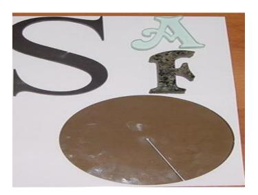
Fig.3. Laser cut examples of technology (glass, composite, stone, sitall)
