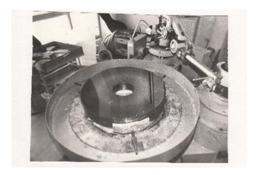
Fig. 4. Big size SiC mirror under polishing
